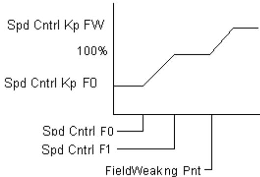
The P gain adjust by speed has two parts associated with it: First, the gain can be modified at lower frequencies, and gain modified above the field weaken range. *Spd Cntrl F0* and *Spd Cntrl F1* define the frequency window which will modify the gain. The block gain will change linearly from the setpoint *Spd Cntrl Kp F0* at *Spd Cntrl F0* to 100% at *Spd Cntrl F1*.
