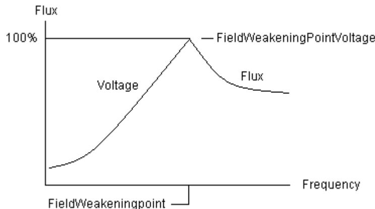
*Id Ref* is adjusted during the field weakened range of the motor. *Field Weakengpnt* defines the frequency to start reducing the motor flux. The drive also monitors motor voltage and reduces the flux to keep the value below *Voltage at FWP*. Another voltage limit is also used to keep the motor voltage below the DC-Link voltage. The motor voltage is limited by *ModIndexLimit* x measured motor volts. *ModIndexLimit* is factory-set to 100%.
