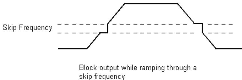
*Freq Reference* is the speed reference after the skip frequency logic in motor Hertz.
