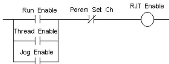
*RJT Enable* is high if any of the modes are enabled and the drive is done with a parameter change. This makes sure all proper values are in place before proceeding.
