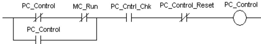
*PC Control* is enabled by the ADDaptACC diagnostic software package. It will transfer into this mode only if the drive is not running. The drive will transfer out of *PC Control* if communications are lost to the computer.
