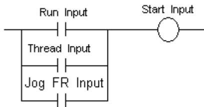
*Start Input* is TRUE when any of the drive run inputs are active.
