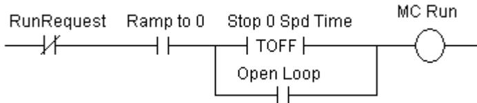
*RunRequest* sets *MC Run* which is sealed in until the drive ramps to zero speed. Also in closed loop mode *MC Run* can be set to stay enabled keeping the drive running at zero speed for *Stop 0 Spd Time* in seconds.
