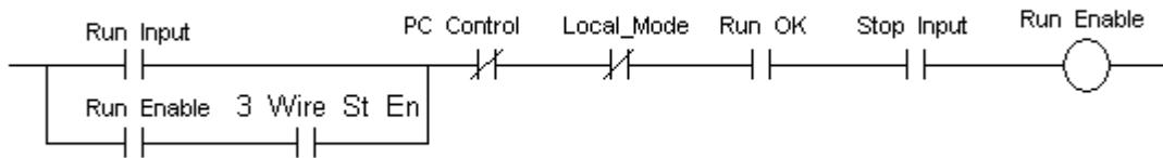
The *Run Input* will energize the *Run Enable* if all interlocks are met.
