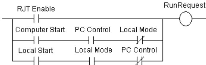
*RunRequest* is high if *RJT Enable* is High or if the drive is commanded to run from either the local mode or computer ADDaptACC mode.
