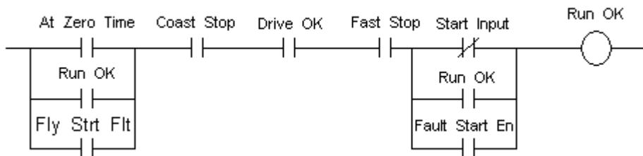
The *Run OK* bit is used to stop the drive in any control mode.
