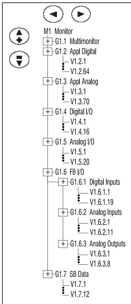
Figure 3-3. Monitor Menu Structure Example
