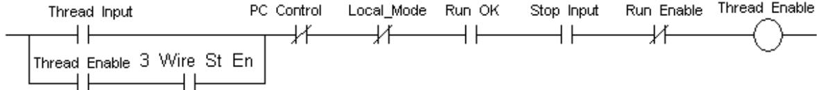
*Thread Enable* is setup similar to the *RunEnable*. *Run\_Enable* takes priority. If in Thread and the *Run\_Input* goes high the control will transfer to the Run mode.
