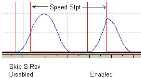
*Disable Ramp* removes both the linear ramp and S-Curve. This should be used only when the drive is a slave section directly coupled and set as a current follower. This works only in the closed loop mode of operation.
