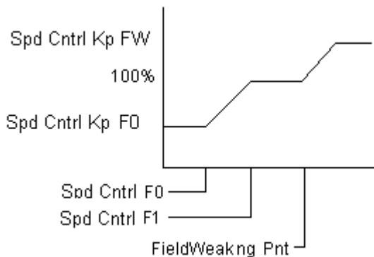
The P gain adjust by speed has two parts associated with it: First, the gain can be modified at lower frequencies, and gain modified above the field weaken range. *Spd Cntrl F0* and *Spd Cntrl*
