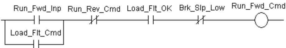
*Run Fwd Inp* is defaulted to the first digital input and provides the run command.
