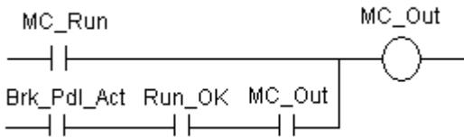
*MC Out* is used to control the motor contactor if available after the inverter. *MC Run* commands the contactor to open or close. *Brk Pdl Act* allows the contactor to remain closed as long as the brake pedal is active. The drive is in coast state with brakes released during this mode.
