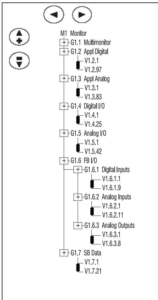
Figure 3-3. Monitor Menu Structure Example
