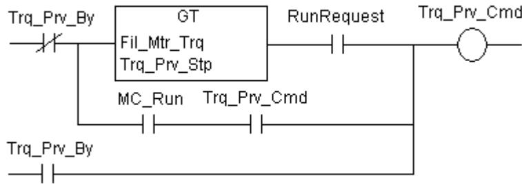
Torque proving is required for hoist sections before the brakes can safely be released. When a run is commanded the drive will run in torque mode and apply torque to the motor. Torque feedback is checked to make sure it is present before *Trq Prv Cmd* goes high and allows the brakes to be removed and the speed to start to ramp.
