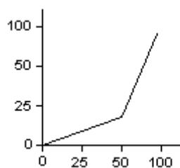
The table provides 20% reference with 50% of the joystick input. It also puts out 100% at 100% joystick input.
