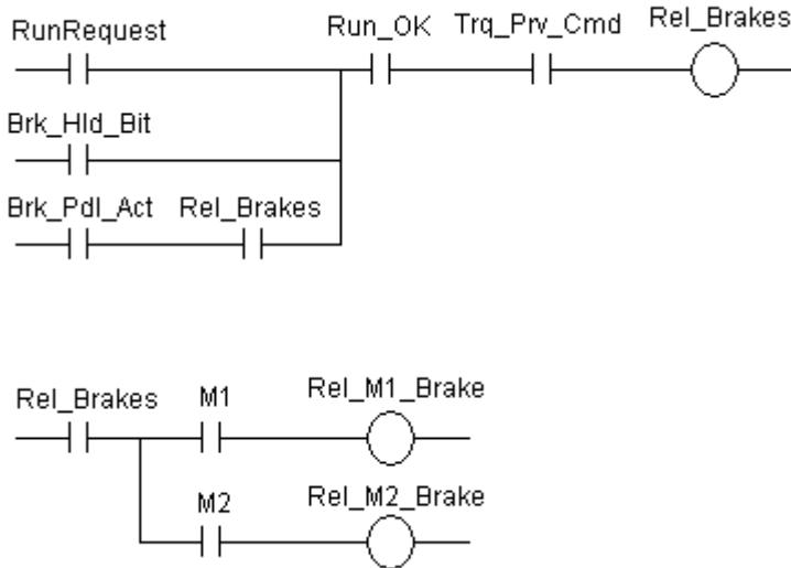
*Rel Brakes* bit is used to control an external motor brake contactor. To use this function it must be configured to a digital output of the drive.
