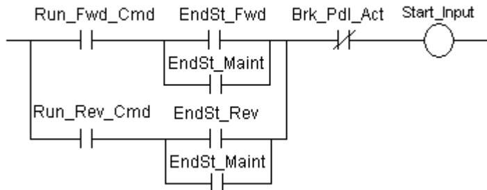
Normally *Start Input* is high when either *Run Fwd Cmd* or *Run Rev Cmd* is active.
