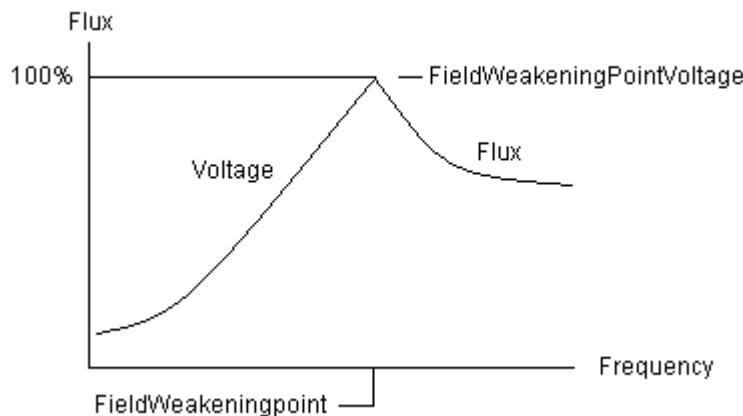
*Id Re Actual* is adjusted during the field weakened range of the motor. *Field Weakengpnt* defines the frequency to start reducing the motor flux. The drive also monitors motor voltage and reduces the flux to keep the value below *Voltage at FWP*. Another voltage limit is also used to keep the motor voltage below the DC-Link voltage. The motor voltage is limited by *ModIndexLimit* x measured motor volts. *ModIndexLimit* is factory-set to 100%.
