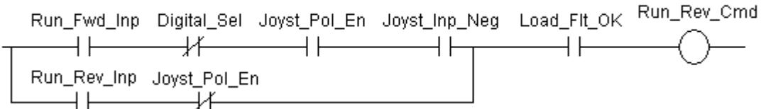
*Run Rev Inp* is defaulted to the second digital input and provides the run command.
