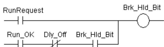
*Brk Hld Bit* is used to keep the brakes from setting until the runs are removed and drive ramps to zero speed. An optional *Brk Open Dly* delay the brakes from setting after zero speed is achieved. Setting the *Brk Open Dly* delay will cause the drive to float the load at zero speed.
