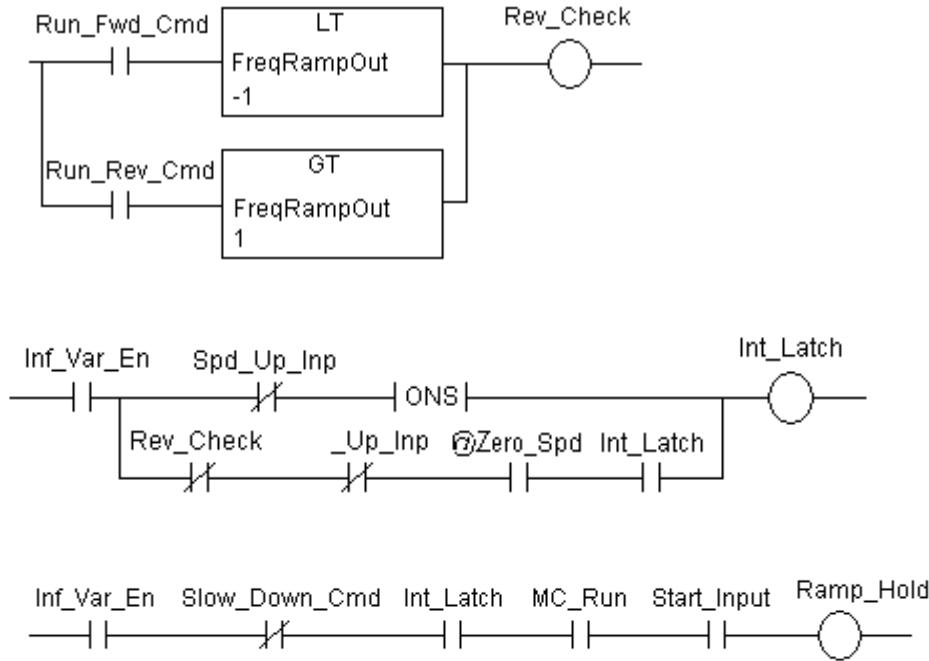
Infinite variable speed control is implemented by having the drive run between zero speed, the first fixed speed, and the second fixed speed. *Run Fwd Cmd* or *Run Rev Cmd* ramps the drive to the first selected fix speed setpoint. When *Spd Up Inp* is selected, the drive will start to ramp to the second fix speed which should be set to maximum speed desired. Removing *Spd Up Inp* will set *Ramp Hold* to stop at the desired speed.
