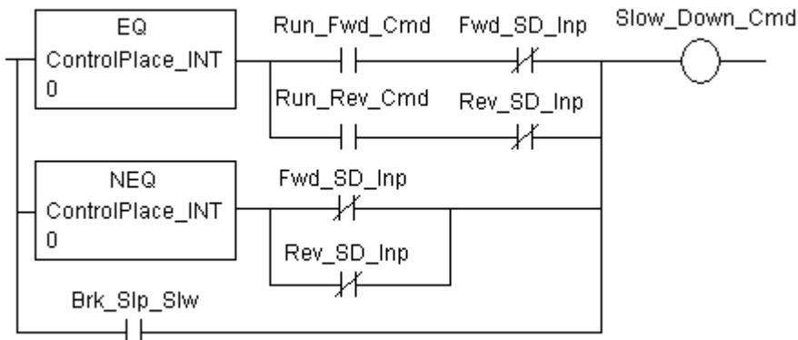
Two separate slow down inputs are available. For safety reasons, these inputs must be normally high and go low during slow down region.
