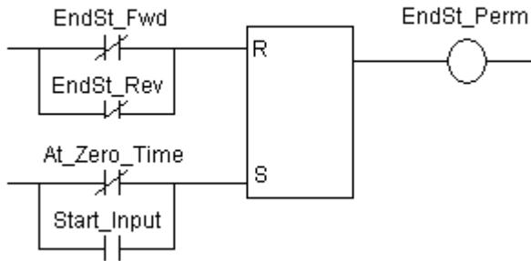
*EndSt Perm* goes high if either of the end stop inputs goes low. It will stay high until the drive has stopped and no run is commanded.
