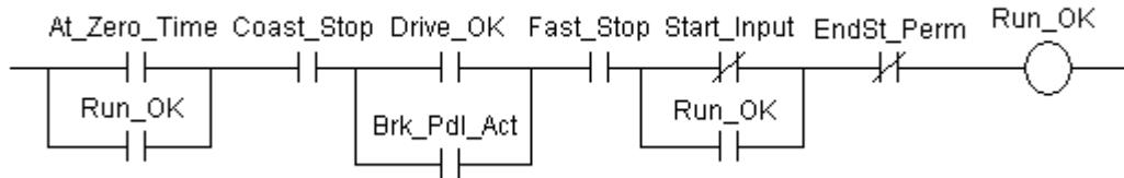
The *Run OK* bit is used to stop the drive in any control mode. The drive will go to a coast stop and the brakes applied.
