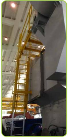
To facilitate field service operations and reduce inspection time, the customer asked Nidec to design the motors with incorporated access stairs ensuring full compatibility with stringent safety standards.
